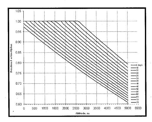
Note: For temperatures in between the specified values in table, correction factor to be considered by nearest temperature value from the Table.
